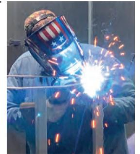
Wherever there is an intersection of metal, we use a full-circumference weld to join the metal together.
