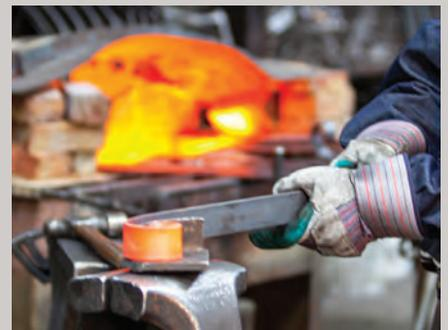
Steel and aluminum pieces are bent into exact shapes and then hand forged with a hammer and anvil, a process unchanged since blacksmiths in the middle ages.
