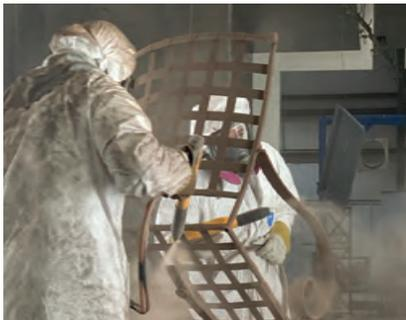
OW Lee employs an extensive process to apply a long-lasting powder coating finish to our frames. Using a chemical reaction, tiny paint-like particles known as “powder” adhere to the frame.
