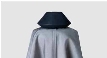
FINIAL The 1.5" x 3.5" finial has a 30% glass-filled nylon interior and HDPE outer shell in a dark grey color.
