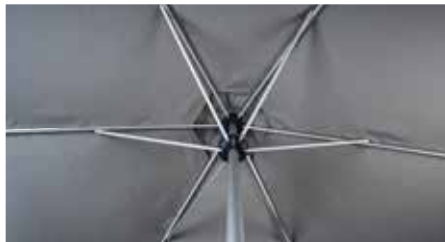
ARMS/RIBS The 3/4" x 1-3/8" arms are non-tapered and are secured to the ribs with stainless steel nuts and bolts.
