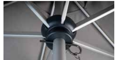
HUB The hub has a 30% glass-filled nylon interior and HDPE outer shell in a dark grey color. It is split horizontally to encapsulate the stainless steel connecting hardware. Six screws secure the hub together.
